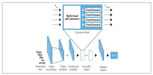
Figure 3-2. Zooming into the encoder layer
