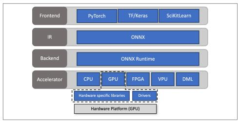
Figure 8-9. Architecture of the ONNX and ONNX Runtime ecosystem (courtesy of the ONNX Runtime team)
