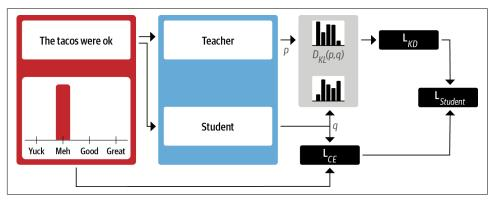
Figure 8-4. The knowledge distillation process
