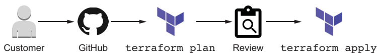
Figure 10.1 Customers make PRs against a version-controlled source repository. This PR triggers a plan, which is reviewed by a management team. When the PR is merged, an apply runs and the resources are deployed.
