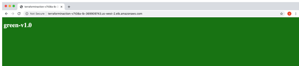
Figure 9.6 The application load balancer currently points to the Green autoscaling group, which hosts version 1.0 of the application.
