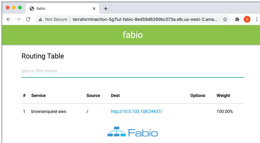
Figure 8.16 After the services are marked as healthy by Consul, they can be detected by Fabio. In AWS, Fabio routes HTTP traffic to the dynamic port that BrowserQuest is running on. In Azure, Fabio routes TCP traffic to the dynamic port MongoDB is running on.
