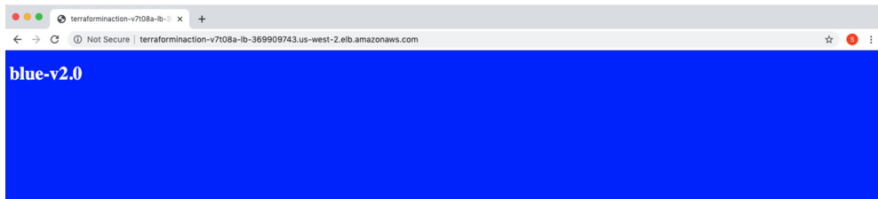
Figure 9.7 The load balancer now points to the Blue autoscaling group, which hosts version 2.0 of the application.
