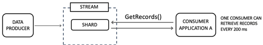
Figure 4.11 – With the GetRecords API, records are pulled by the consumer
