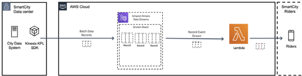
Figure 4.20 – City data system emergency message producer and AWS Lambda consumer
