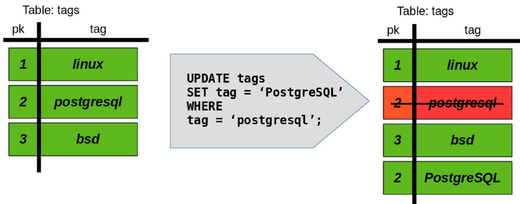
Figure 11.1: Updating a tuple creates a new tuple and invalidates the old one
