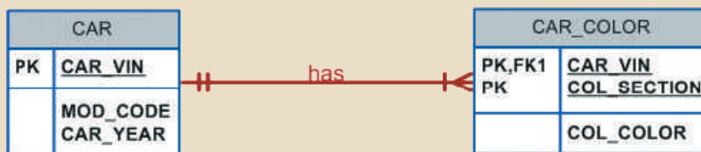
FIGURE 4.5 A NEW ENTITY SET COMPOSED OF A MULTIVALUED ATTRIBUTE'S COMPONENTS
