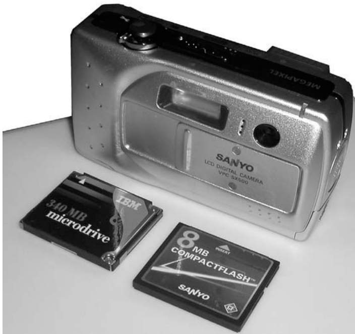
FIGURE 8.14 The Sanyo VPC-SX500 with Flash memory card and IBM Microdrive. Although newer cameras offer more pixels per picture, the principles are the same. This 1360 × 1024 pixel digital camera stores pictures either using CompactFlash memory or using a IBM Microdrive. This photo was taken using a 340 MB microdrive and a 8 MB CompactFlash memory. As Figure 8.15 shows, in 2004 the capacities are as large as 1 GB to 4 GB. It is 4.3 inches wide × 2.5 inches high × 1.6 inches deep, and it weighs 7.4 ounces. In addition to taking a still picture and converting it to JPEG format every 0.9 seconds, it can record a Quick Time video clip at VGA size (640 × 480). One technological advantage is the use of a custom system on a chip to reduce size and power, so the camera only needs two AA batteries to operate versus four in other digital cameras.
