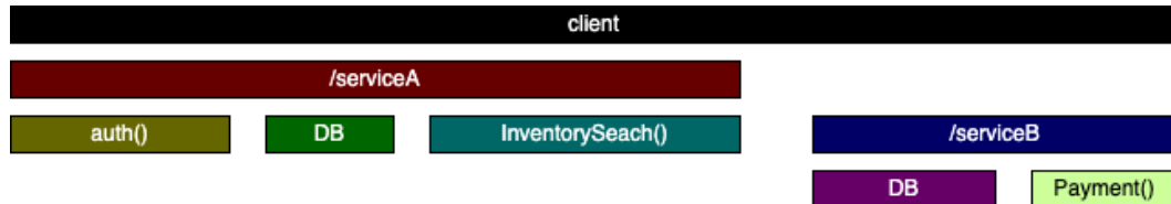
Figure 9.2 – Example of a trace representation using a waterfall diagram
