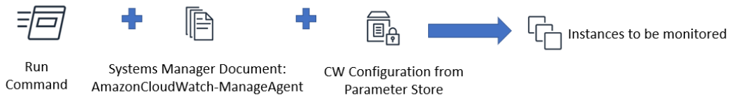
Figure 3.30 – Process to start the CloudWatch agent using AWS Systems Manager
