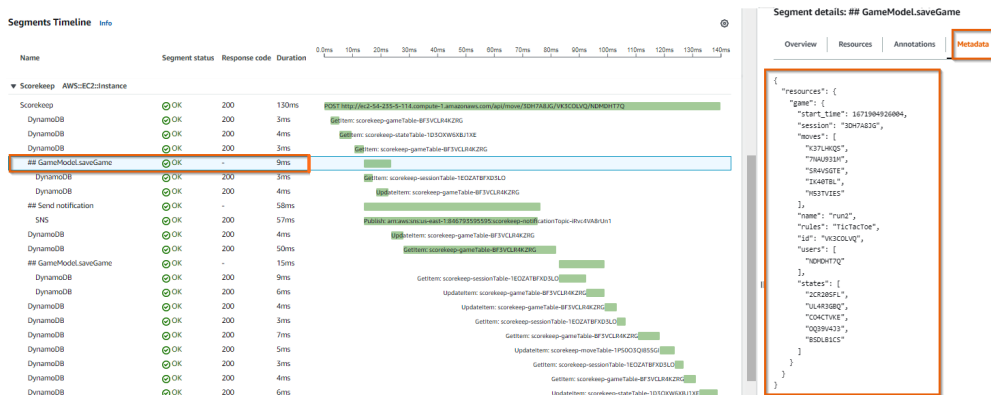
Figure 4.32 – An HTTP POST request highlighting the GameModel.saveGame subsegment and metadata
