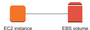
Figure 8.1 EBS volumes are independent resources but can only be used when attached to an EC2 instance.
