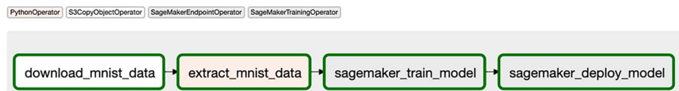
Figure 7.5 Logical steps implemented in Airflow DAG
