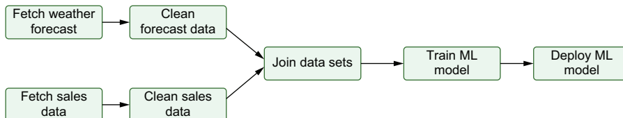
Figure 1.6 Independence between sales and weather tasks in the graph representation of the data pipeline for the umbrella demand forecast model. The two sets of fetch/cleaning tasks are independent as they involve two different data sets (the weather and sales data sets). This independence is indicated by the lack of edges between the two sets of tasks.
