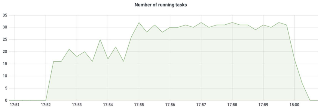
Figure 12.15 An example visualization of the number of running tasks. Here, the parallelism had the default value of 32, to which we sometimes see the number of tasks spike.
