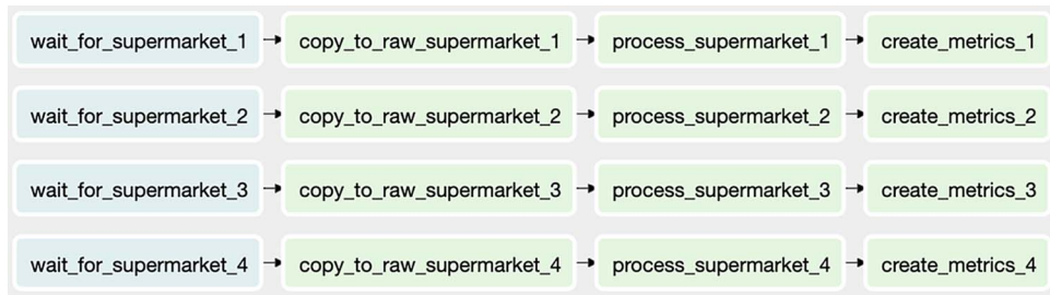
Figure 6.11 Replicating tasks to avoid waiting for completion of all processes
