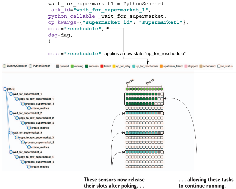
Figure 6.9 Sensors with mode="reschedule" release their slot after poking, allowing other tasks to run.
