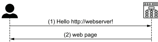
Figure 13.14 With HTTP, the validity of the caller is not checked, and data is transmitted in plain text.
