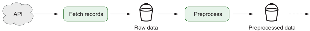
Figure 11.7 Storing intermediate data from tasks ensures that each task can easily be rerun independently of other tasks. In this case, cloud storage (indicated by the bucket) is used to store intermediate results of the fetch/preprocess tasks.
