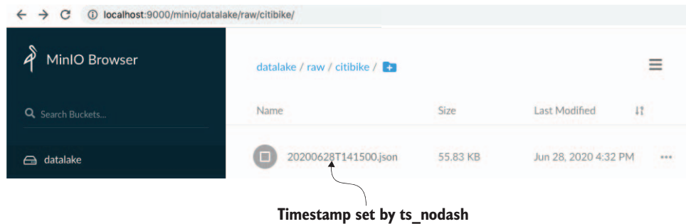
Figure 14.5 Screenshot of the MinIO interface showing a file written to /datalake/raw/citibike , and the filename templated with ts_nodash .
