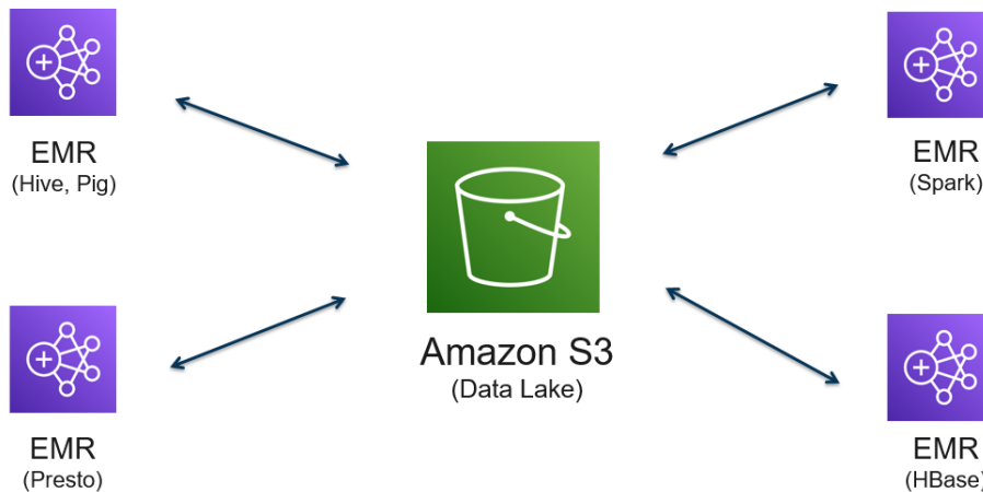
Figure 1.3 – Multiple EMR clusters using Amazon S3 as their distributed storage
