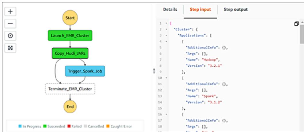
Figure 12.1 – AWS Step Functions visual workflow for EMR jobs
